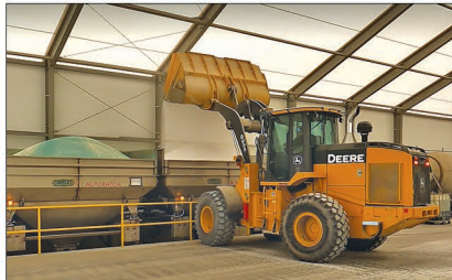
Reclaim and loadout can be controlled from a loader tablet to maximize the operator's time.
