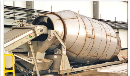
Kahler system controls 16-ton rotary blender plus conveyors, scales, discharge gates & more.
